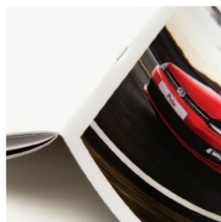
The most cost effective method of binding one or more printed sections together, with or without a cover, by means of wire stitches through the spine and centrefold. A saddle-stitched document must be at least eight pages long and increase in length in four-page increments. Saddle-stitching is suitable for documents of up to around 80 pages.
