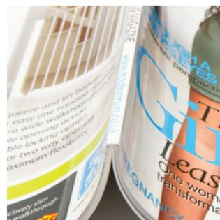
Perfect Binding is often chosen when the number of pages makes the document too thick to saddle-stitch or for aesthetics. The pages and printed sections are gathered in order, spine milled and held together with a hot melt adhesive. A cover (usually on a heavier paper weight) is attached to the spine and is formed around the book.
