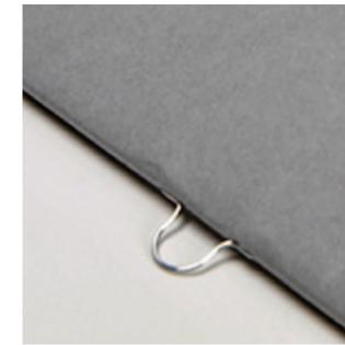
This is a method of saddle stitching whereby the stitch is formed into a semi-circular loop that sticks out beyond the spine of the publication. These loops slip over the rings of a binder serving as an alternative to hole punching.
