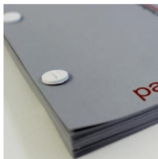
Used for binding loose sheets. Pillar and post screws are used to secure the printed document. The pages are gathered in order, drilled, and the pillars and posts are inserted until they meet - they are secured by screwing the pillar and post together by hand. Pages can be added in two page increments.
