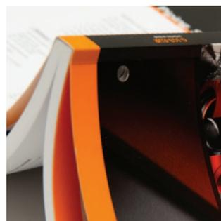
PUR binding is similar to perfect binding and looks the same in appearance, but uses a more durable and flexible glue. It is chosen for its lay flat qualities and the strength of the bind. It is nearly impossible to remove pages from a PUR Bound book, it is approximately 30% stronger than a standard perfect bound book and the spine doesn't deteriorate with age. It is ideal for printed items that need to be durable reference tools.
